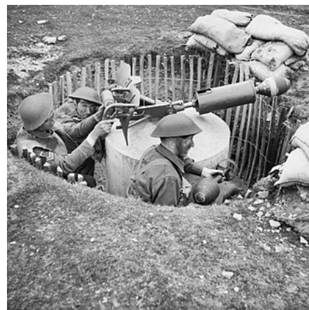
Home Guard soldiers training with a Blacker Bombard anti-tank mortar in May 1943. The mortar is mounted on a concrete pillar in a pre-prepared pit; of which around 18,000 were dug
